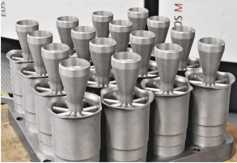
Figure 4 Production of more than 1000 gas turbine swirlers per year with qualified industrial production process at Siemens Energy [26]. Picture courtesy Siemens Energy.
