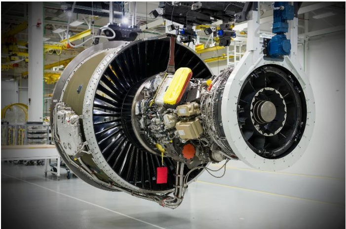
Figure 7 Pratt & Whitney aeroengine PW1500G/PW1900G with fan case mount ring manufactured by DED-LB/wire by GKN Aerospace [36]. Picture courtesy GKN Aerospace
